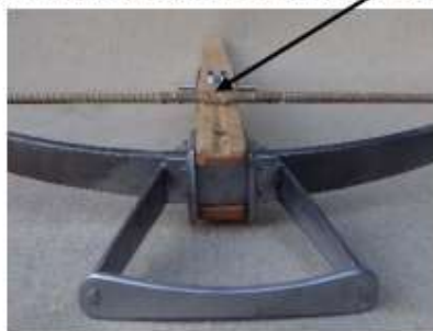
Lath (prod) assembly below Bolt track.
